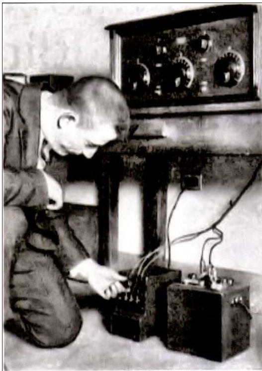
Fig. 3— Simple installation of a B battery eliminator. Simply connect wires between the binding posts of the radio receiver and those of the eliminator, and plug the eliminator into wall socket. At right is seen the A battery. A cable holds all leads for battery and eliminator.
